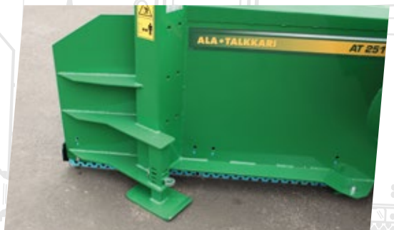
Perforated grader blades and adjustable supports are included as a standard (AT-251 26.)
