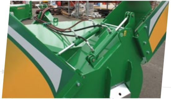
The hydraulic snow hatches have hinges on top that allow you to control the flow of snow (AT-251 26 pictured).
