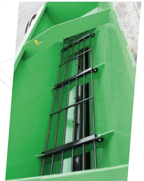
The crusher efficiently prevents blockages in the sand spreader.
