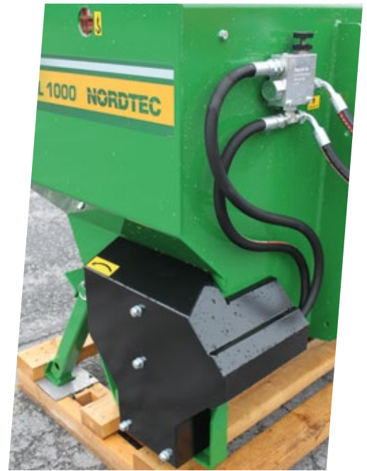
The upwards widening design of the dipper protects the machinery and device controls.
